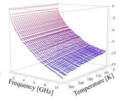
Round trip RF attenuation as a function of connector temperature
